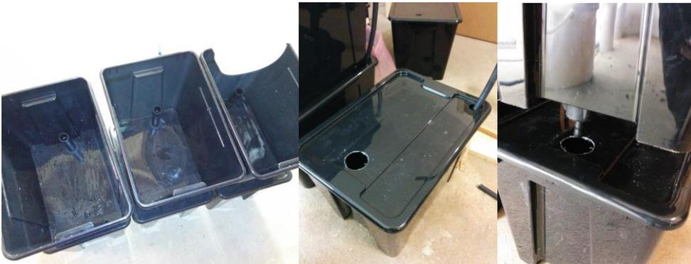
**Figure 2:** From left to right: Adding the bulkhead fitting + standpipe to the grow bed component, drilling the bulkhead fitting hole and pump hose in the support lid of the grow bed and a close-up of the bulkhead fitting being inserted in the lid hole.
