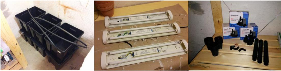
**Figure 1:** From left to right: The three container units with the plumbing tubes, the three light fixtures, and the three pumps, connectors, standpipes, and bulkhead fittings.
